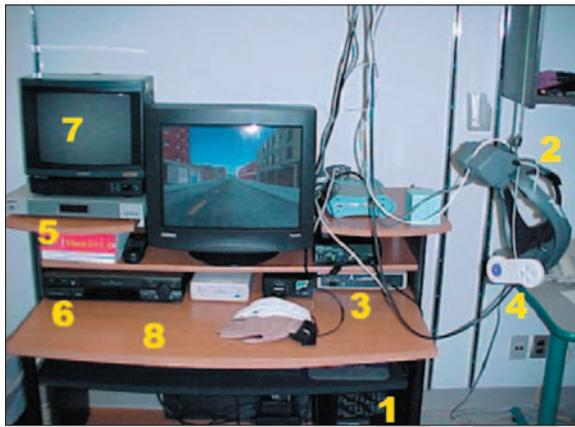
**Figure 1.** Layout of the equipment used to conduct this virtual reality experiment (see text for explanation of functionality of each component). 1. ZX-10 Intergraph Computer Workstation. 2. Proview XL-50 Head Mounted Display. 3. miniBird 800 6 Degree-of-Freedom tracker. 4. Joystick. 5. Sony Scan Converter. 6. Mitsubishi Video Cassette Recorder. 7. Sony TV monitor. 8. Movable desk unit.
